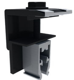
Image 2.4.10-1 Universal end clamp w/WEEB-BMC [96 in-lbs (11 N-m)]
